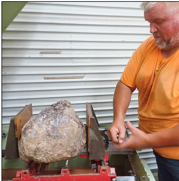
Serious Slabbing with a Rock Saw at the SNGMS Lapidary Shop
